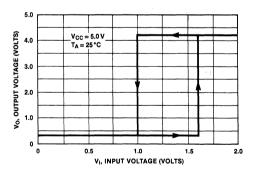
Figure 9. Typical Bus Load Line
